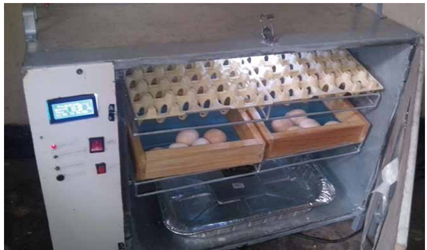
The Egg Incubator uses technology to simulate the natural process whereby a hen sits on eggs and hatches them in an artificial environment.
